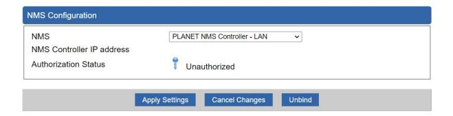
Figure 4-4-23 NMS Controller – LAN Configuration Page
