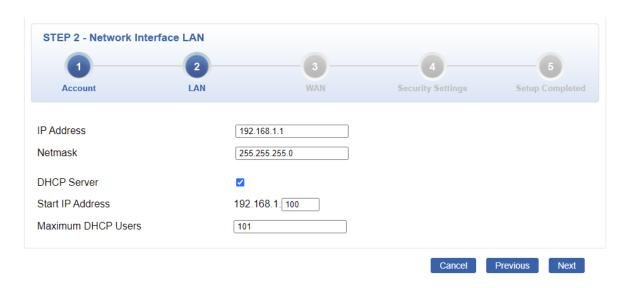
Figure 4-4-4: Setup Wizard – LAN Configuration
